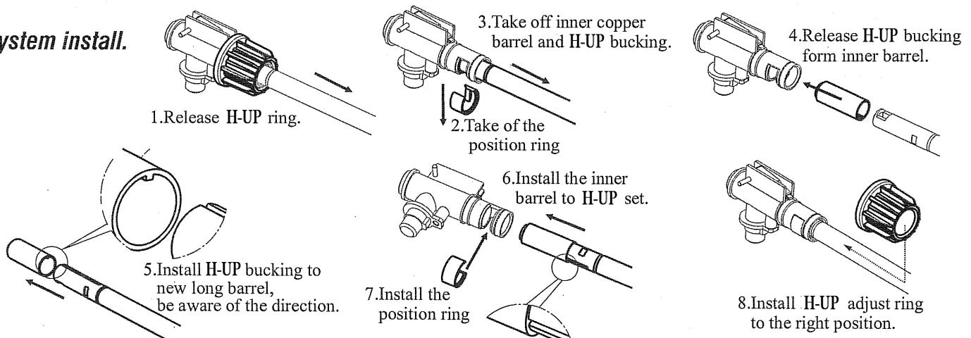
**Barrel system install.**
