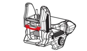
將調整扭轉左即可升高準星；將調整扭轉右即可降低準星。 Rotate the dial counterclockwise to raise the aiming point. Rotate clockwise to lower the aiming point.
