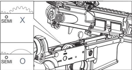
3號齒在槍身結合時，必須轉到正確位置，才可將上槍身蓋下。 Make sure the sector gear is turned to the correct position before reassembling the receiver.
