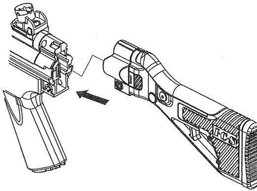
3 Insert the pin to finish installation
