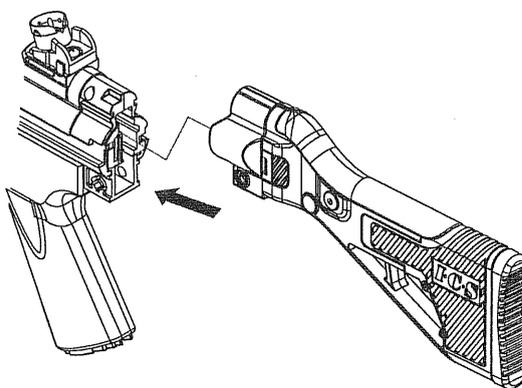
3 Insert the pin to finish installation
